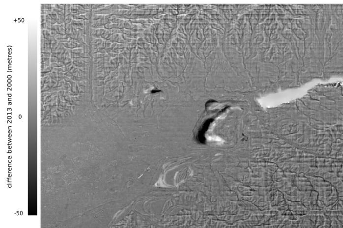
Fig. 4. Difference between DEM from Pleiades (2013) and SRTM (2000) over Angren, Uzbekistan – difference in landslide areas goes up to 50 m affecting InSAR detection ability (Lazecký et al., 2013)
